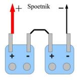
In some cases 2 x 4 Battery holders are supplied with the kit. If so, please connect them in serial connected like the picture .
