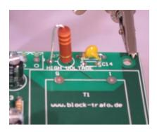
Now it's time for the larger / higher parts. You can now assemble the volume potentiometer (POT1) and R7. R7 is mounted upright. Bend this wire all the way around, past the body's resistance. Now you can mount the resister straight up . Insert the straight wire through the hole in the circle. The other wire comes into the adjacent hole.
