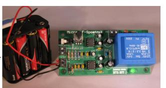
The construction of the Sputnik is the same principle as the construction of regular self-build packages. It starts with the parts that are the lowest from the board. Then the higher components. In this building description, a preferred construction sequence is given.
