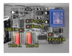
The external contact (P4) can be used to switch contacts, for example, a momentary short circuit greeting card. Often this requires a short pulse for a tune to continue playing. The speed of these pulses will be determined by the "trigger".
