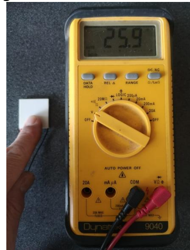
Measurement of the tension of the Peltier element. Left: voltage about 0 Volts, middle: voltage negative, right: voltage positive.
