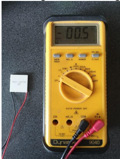
Measurement of the tension of the Peltier element. Left: voltage about 0 Volts, middle: voltage negative, right: voltage positive.
