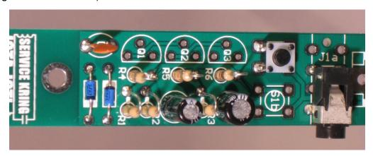
Transistors: 3 x BC547C (note the flat sides!)
